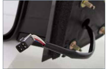
110988 & 110989 - Power 4-way Mirror: Power, adjustable mirror with manual fold-away feature with OE style connector plug
